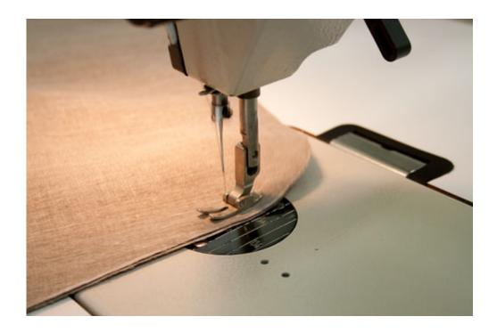
Attach the two pieces together by seaming along all the edges except for the top opening.
